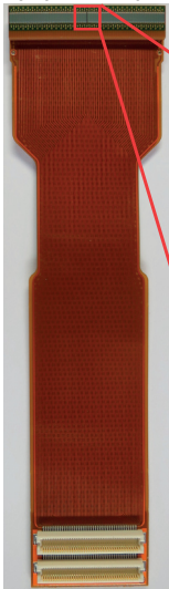
SiPM array with flex cable and connector 32.54mm x 12cm
