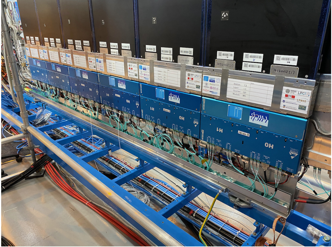
Figure 5.5: Photograph of six ROBs mounted on the bottom half of a C-Frame and ready to be commissioned.
