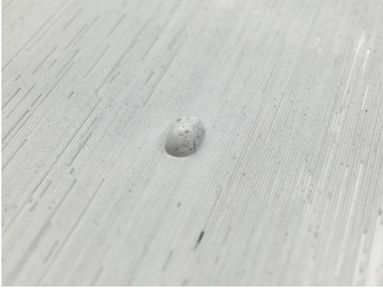
Figure 3.9: Close-up view on a wound fibre mat with alignment pin. Image taken from Ref. [50].
