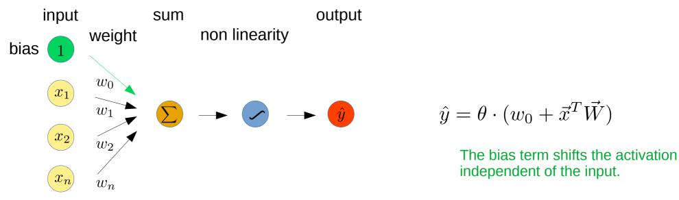
Idea: minimize a cost function to determine the weights and bias of the perceptron by comparing the predicted output and the true output.
